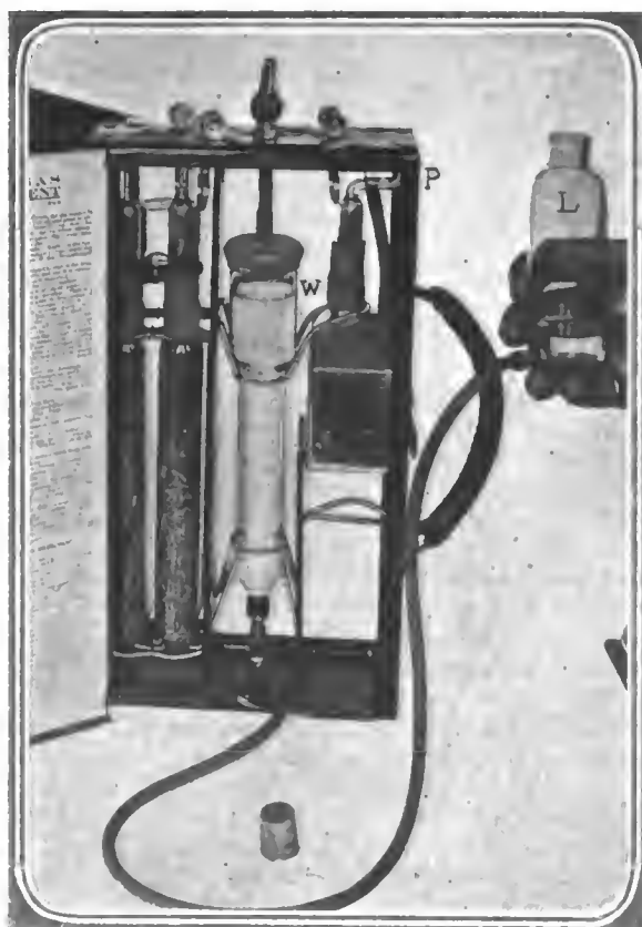
Fig. 4—Filling the burette with acid water. For this purpose the cock is turned open and the leveling bottle raised as shown in the picture. This operation is also used when it is necessary to coax the caustic into the chamber.
